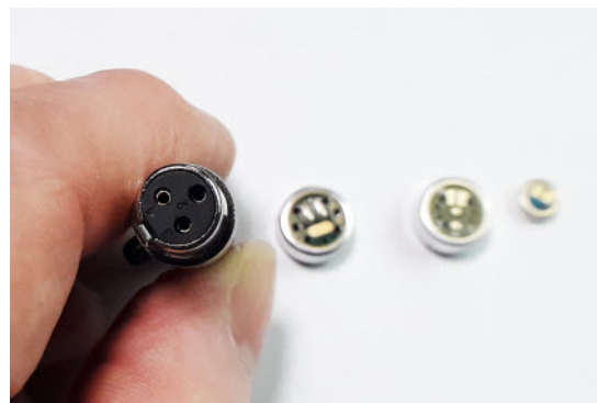
Converting a 3-wire connected mic to 2-wire will produce a 10db increase in gain - but usually at the expense of turning the signal into a -ve phase signal
