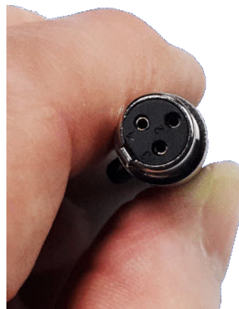
Lavalier mics terminated with a multipin plug will output a normal positive phase signal
